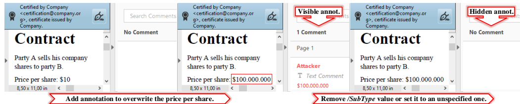
Figure 4.1: A certified document. The Price per share was manipulated by a FreeText annotation to show the value $100,000,000. The PDF viewer displays this annotation in UI-Layer 3. By deleting the /Subtype value the PDF object, it can be removed.
